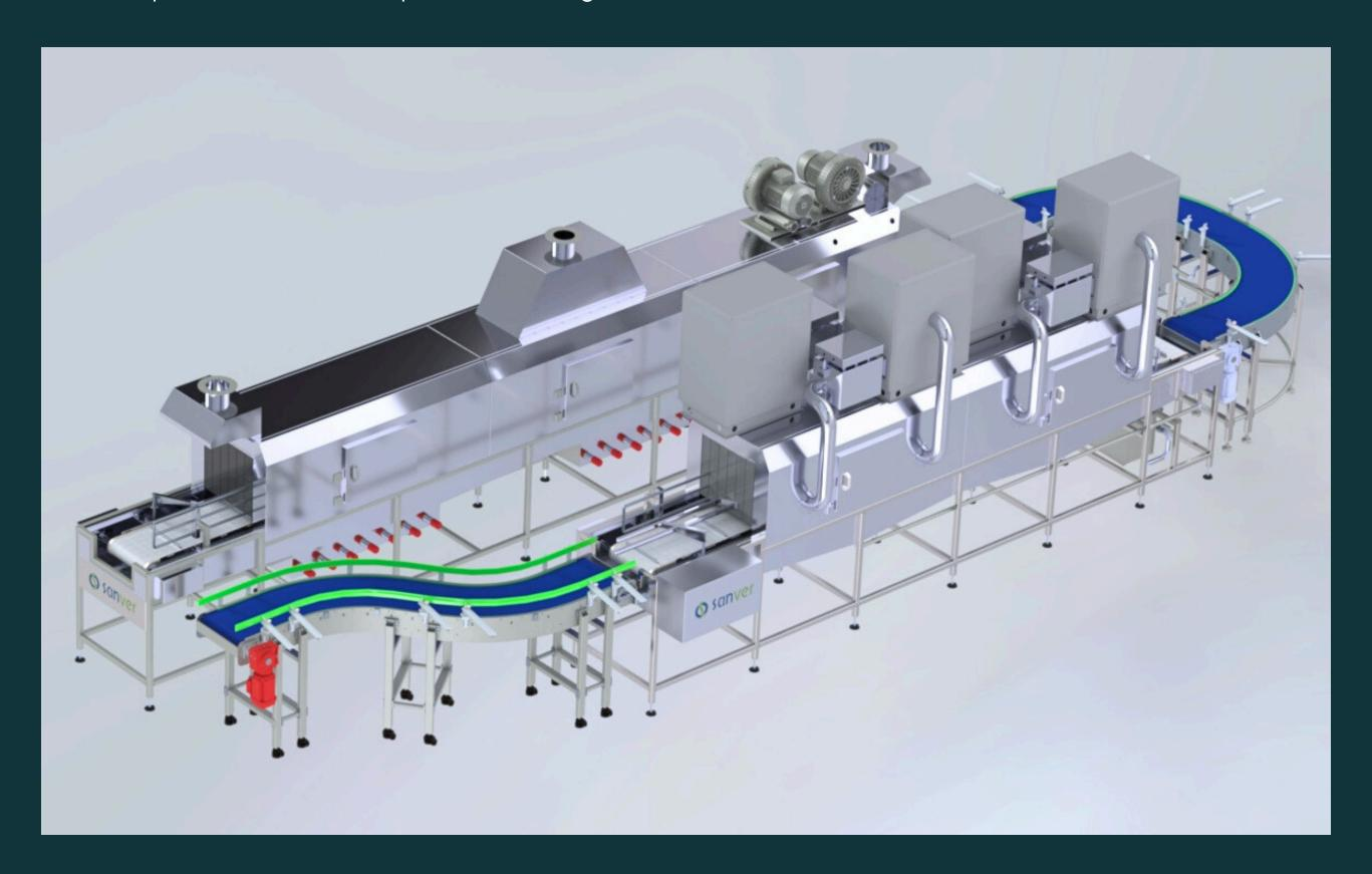
The system features a multi-stage washing structure that can be configured based on product requirements. Each module operates independently with its own circulation line and filtration system.
